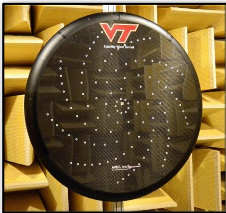
117-microphone phased array
